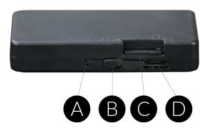
A – Reset button B – Power switch C – Micro SD card slot D – MicroUSB power socket
