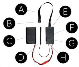
A – Flex cable B – Pinhole lens C – Battery
